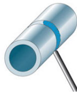
PG Pipe: fixed Axis: horizontal ASME: 5Gd
