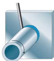
PB Pipe: rotated Axis: horizontal ASME: 2F
