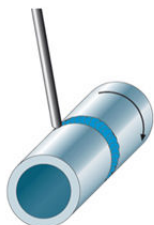
PA Pipe: rotated Axis: horizontal ASME: 1G
