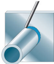
PF Pipe: fixed Axis: horizontal ASME: 5Fu
